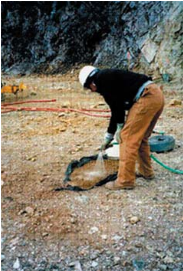
Figure 5-11. Spray application of the material sent to MLI for HC testing.
