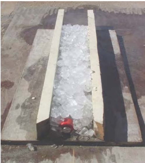
FIGURE G-1. A soil core capped and cooling in an ice bath. The thermometer is visible in the end cap.
