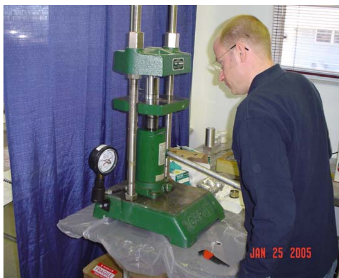
Figure 6-2. Oxford ED2000 soil pellet sample preparation.
