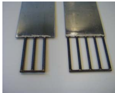
Photo 1 Box Type Filling Unit and Flow Obstacle
