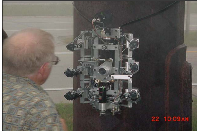
Figure 31. Remotely Operated Inspection Device.
