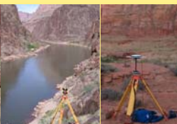
GPS Technology or Conventional Survey methods are used to geo-reference Control Points.
