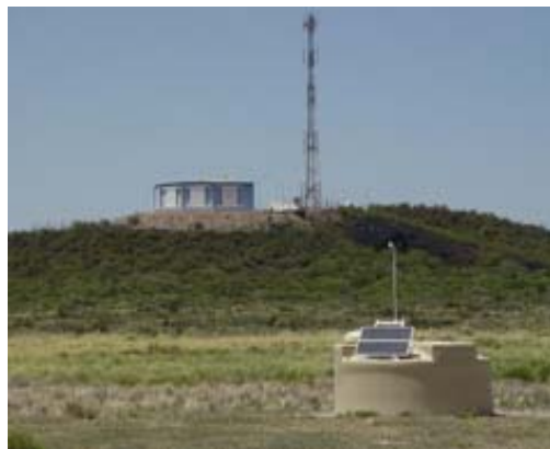
The Los Leones Fluorescence Detector together with its closest Surface Detector tank. Credit: Pierre Auger Observatory.
