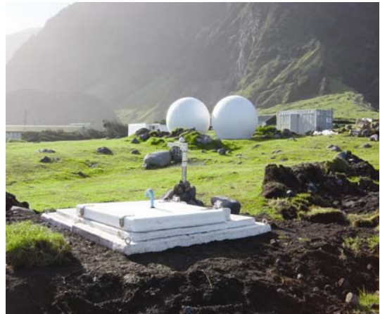
This is an image of the entrance to the Global Seismic Network's seismic vault on Tristan da Cunha in the South Atlantic. This station is part of a collaboration with the Comprehensive Test Ban Treaty Organization International Monitoring System and Geoscope. Credit: Ted Kromer.
