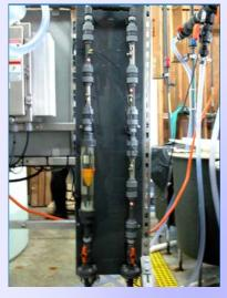
Prototypic Treatment Technology at USGS Marrowstone Marine Field Station. Three electrolytic cells are used to generate hypochlorite from seawater (NaCl). Each cell consists of a cathode and an anode.
