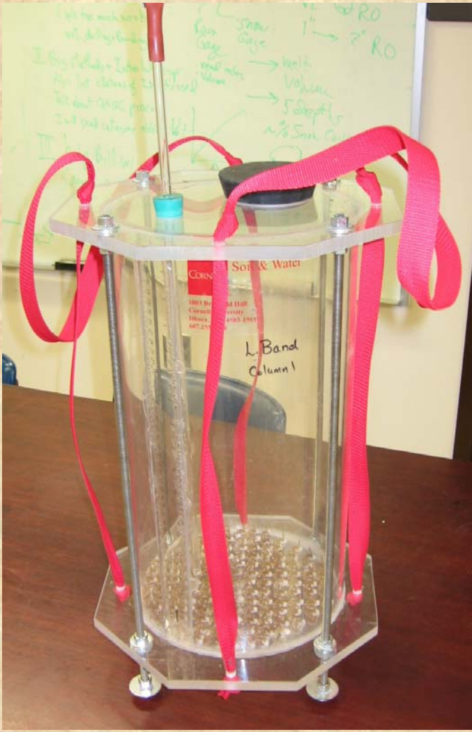
BES: Cornell Infiltrometer
