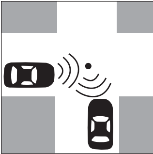
Intersection Collision Warning
