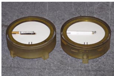
Reduced-ignition propensity test method (ASTM E2187) developed by a team led by Richard Gann of the Fire Research Division, and adopted by the States of New York, Vermont and California and the Dominion of Canada to reduce cigarettes as an ignition source for fires.
