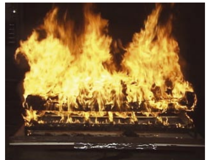
Example of fire growth on a bed incorporating an unimproved mattress.
