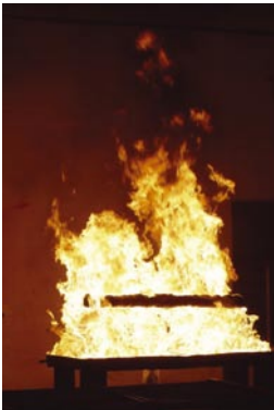
2.0 MW heptane fire from liquid spray burner.
