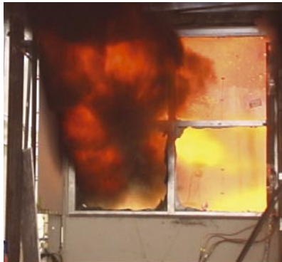
Response of glass-based partition to a real-scale fire.
