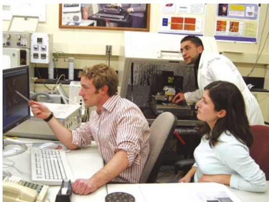
BFRL researchers using atomic force microscopy to characterize the nanoscale morphological properties of pigmented polymeric coating films.
