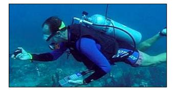
In collaboration with the NPS, USGS developed monitoring protocols (in use in the Virgin Islands and Dry Tortugas) that use video cameras, sonar, and GPS to document reef changes and ensure precise and accurate locator information (contact: Caroline Rogers).
