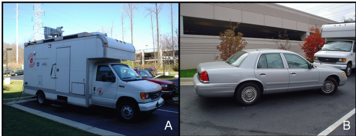
Figure 1 – (Left, 1A) The Mitretek Mobile Wireless Laboratory (MoWL). The 999J IR sensor can be seen facing downward on the front bumper. (Right, 1B) The blue 1998 Ford Crown Victoria. This was one of two similar passenger vehicles used to collect temperature data during the project.
