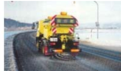
sprinkling anti-freezing agent
