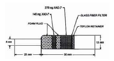
Figure 1. OVS-7 Sampling Device
