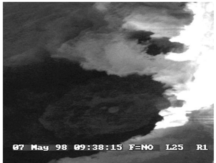
Figure 13. Infrared video image of roil between two warm-water plumes, showing slightly warmer water in center beginning to spread out radially. White area is hot; ocean entry to right. Video taken May 7, 1998.
