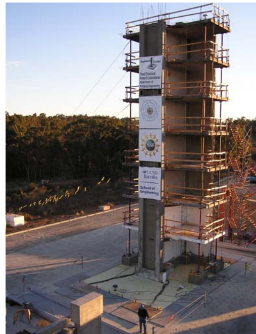
Researchers at the University of California, San Diego, in partnership with industry, use the largest outdoor shake table in the U.S. as part of NEES to test the tallest building structure ever on a shake table. This seven-story, 65-foot tall, reinforced concrete structure is being tested to investigate "promising new designs that might improve the earthquake safety of apartment and condominium buildings and other residential structures in densely populated and seismically active regions in Los Angeles and Southern California." Credit: Professor José I Restrepo, Department of Structural Engineering, University of California, San Diego
