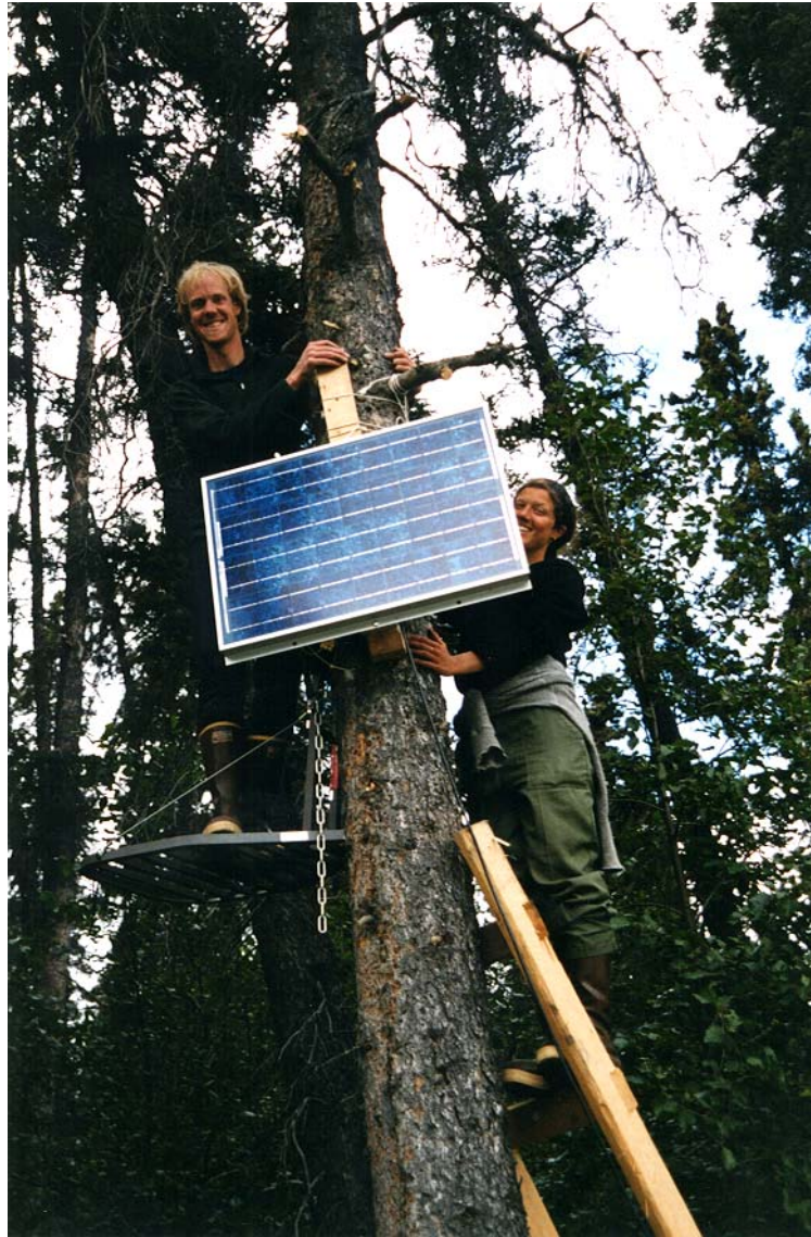
Figure 2. Dan Young and Rita Cochran install a remote solar-powered telemetry receiver and antenna. As radio tagged salmon pass the site, the receiver identifies which fish passed at what time and day.
