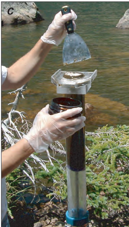
Figure 6. (A) Transport of sediment sampling gear to a lake in Glacier National Park, (B) crew working from an inflatable boat, and (C) collection of surface sediment from lake core.
