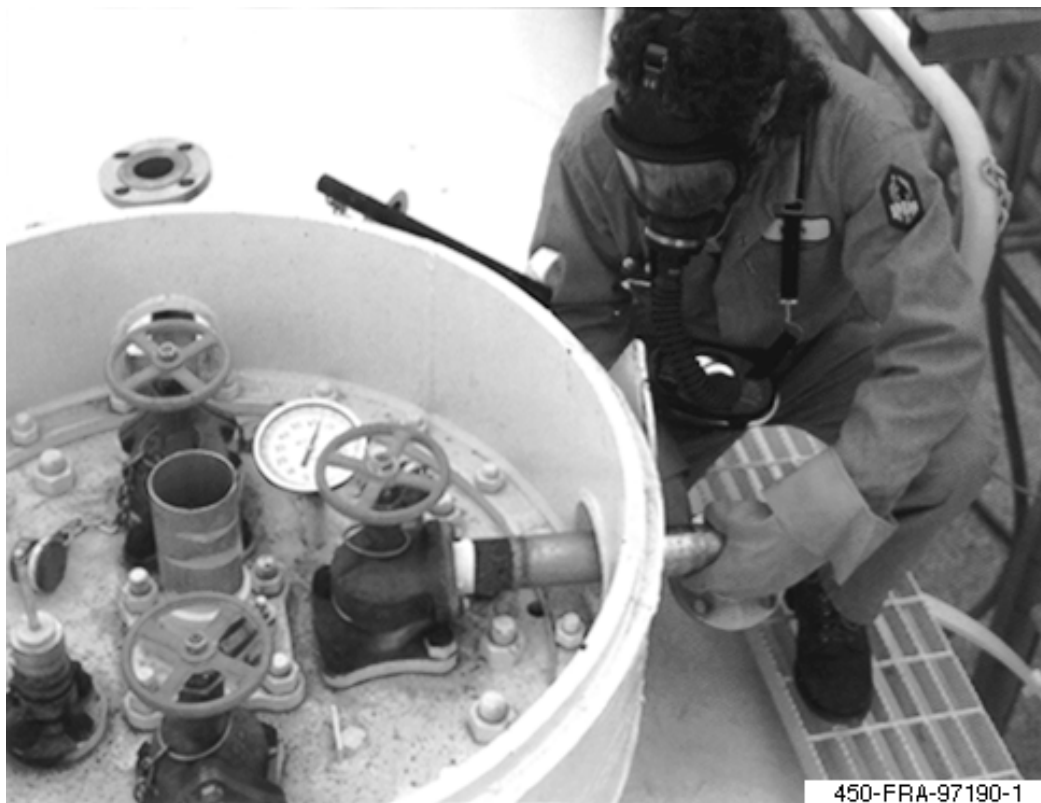
Figure 5. Respiratory protection equipment is required when unloading ethylene oxide
