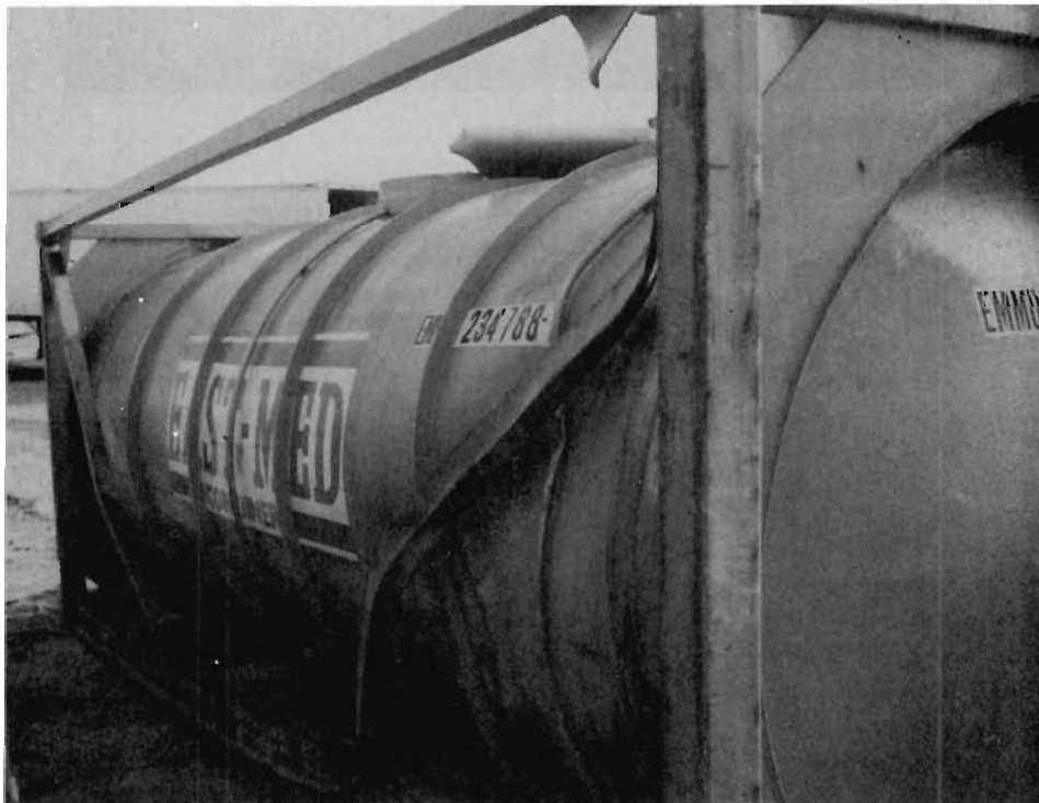
FIGURE 5-28 DAMAGE TO IM 102, EMMU 234788-7, LOCATION 2B (COFC), ACCORDION TEST
