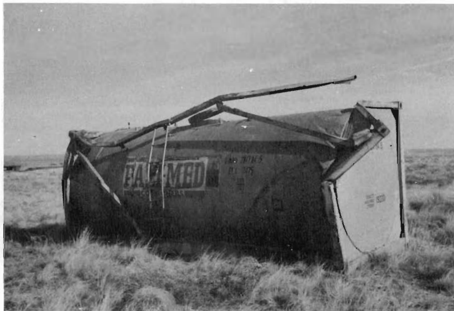
FIGURE 5-25 DAMAGE TO INSULATED IM 102, EMMU 234784-5, POSITION 1B (TOFC) ACCORDION TEST
