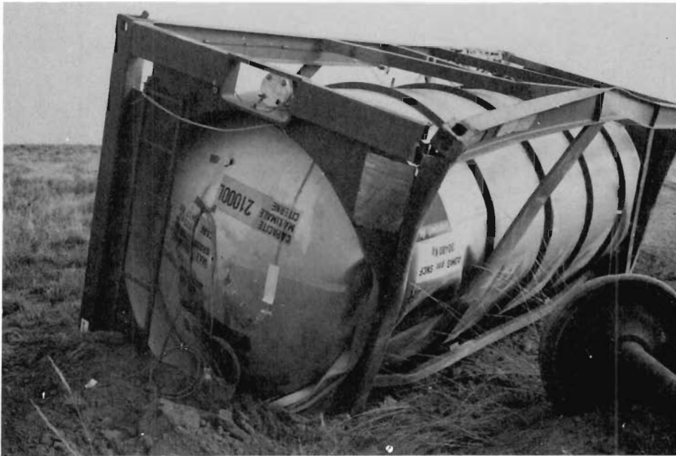
FIGURE 5-21 DAMAGE TO BLSU 300019 AFTER BROKEN RAIL DERAILMENT TEST 3 (ALSO USED IN TEST 1) AT 42.0 MPH
