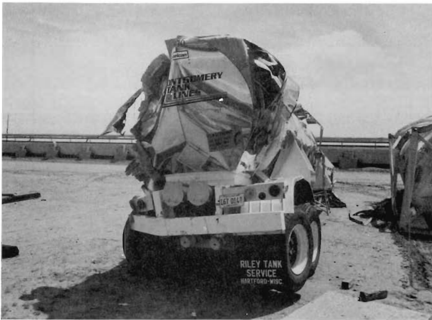
FIGURE 5-8 MC 307 MTLZ 6970 TANDEM END VIEWS OF DAMAGE AFTER THREE BROKEN RAIL DERAILMENT TESTS
