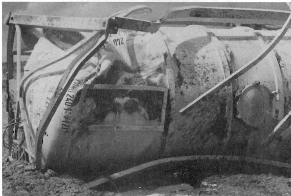
FIGURE 5-23 DAMAGE TO PORTABLE TANK IN BROKEN RAIL DERAILMENT TEST 5 AT 64.5 MPH
