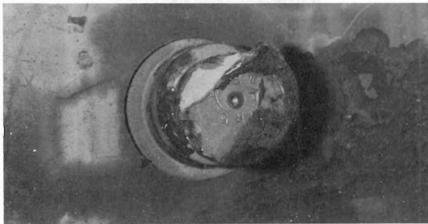
FIGURE 5-7 MC 307 FAILED KINGPINS
