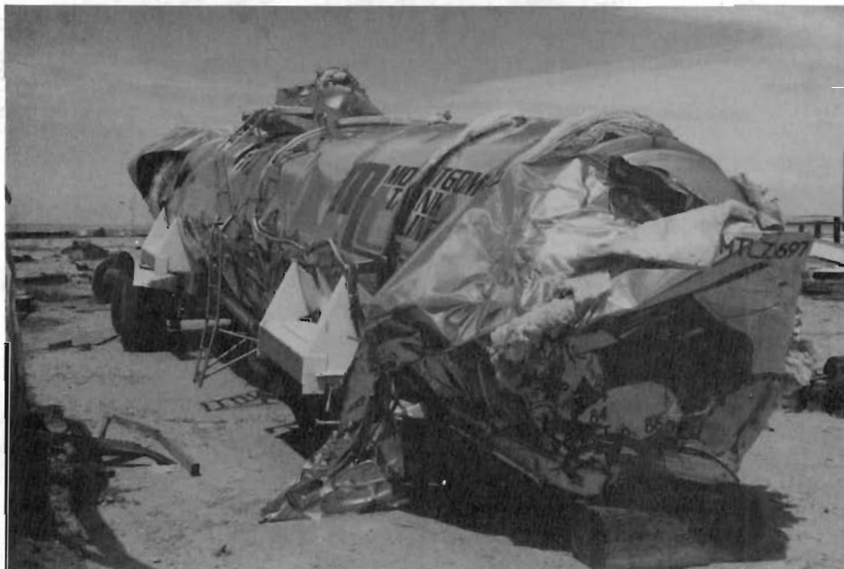
FIGURE 5-9 MC 307 MTLZ 6970 HITCH END VIEWS OF DAMAGE AFTER THREE BROKEN RAIL DERAILMENT TESTS
