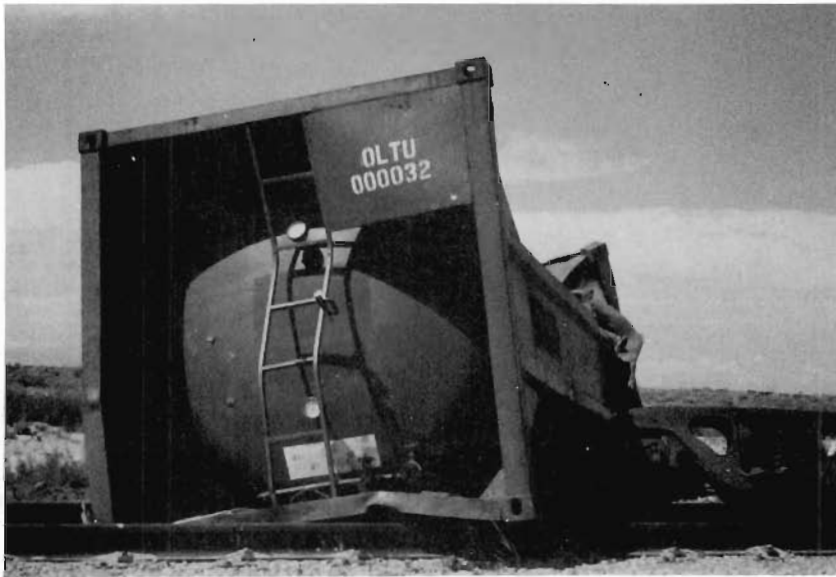
FIGURE 5-24 DAMAGE TO PORTABLE TANKS IN BROKEN RAIL DERAILMENT TEST 6 AT 59.5 MPH
