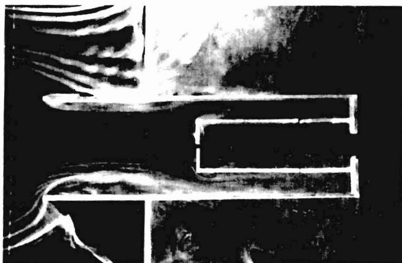
Figure 5.2 Visualization of Blocking Effect Due to Valve in Flow Rate Measurement Nozzle
