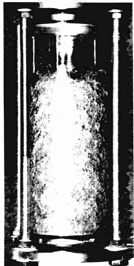
Figure 4.7 Continued Heavy Pool Boiling - Large Exit Orifice (medium: Freon 12)
