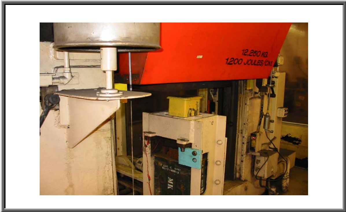
Figure 20. 27,000-lb hammer over test setup
