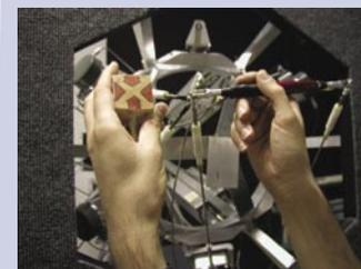
A bimanual haptic interface developed at the University of Colorado at Boulder enables users to move and manipulate virtual objects easily with both hands. The "cube" has a 6-degree-of-freedom position sensor that allows the user to position virtual objects precisely so that he or she can then "operate" them with the actively force-controlled 6-degree-of-freedom "stylus."
