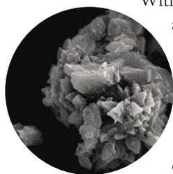
With support from NSF, researchers at NanoScale Materials, Inc., developed scaled-up production processes for FAST-**ACT** (First Applied Sorbent Treatment Against Chemical Threats), an advanced nano-engineered family of products designed to provide first responders, hazmat teams, and other emergency personnel with a single technology to counteract a variety of chemical warfare agents and toxic industrial chemicals.
