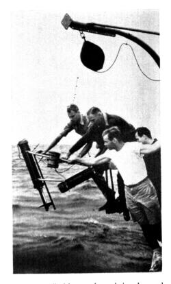
The recently constructed "luminescence camera" (shown above being lowered from an oceanographic vessel) is activated when the flash of an animal that swims or drifts into the sensitive region of the instrument is picked up by the shielded photomultiplier tube. The large and rather rare medusa shown below was photographed at a depth of 1,000 meters off the eastern tip of Georges Bank.
