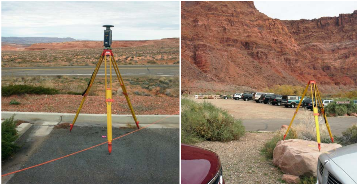
Figure 2-1 FPI GPS Base Stations: PAG1 (left) and LES1 (right)
