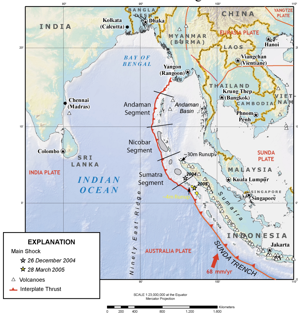
Fig. 1. Regional map of Sumatra and the Bay of Bengal, showing the epicenters (stars) and regions of high slip for the December 2004 earthquake (gray, representing regions of slip >10 m) (Chlieh et al. , 2005) and March 2005 earthquake (yellow, representing regions of slip >5 m) (Ammon et al. , 2005; Ji, 2005). For descriptive purposes, the December 2004 rupture is broken into three segments: Sumatra, Nicobar, and Andaman.
