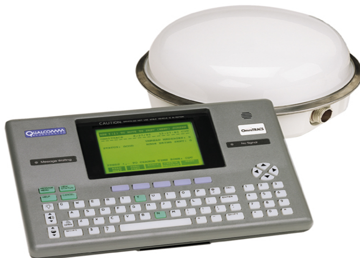
Figure 7: Tractor Mobile Communications Terminal
