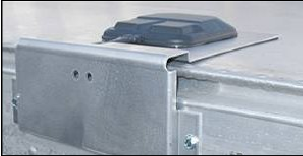
Figure 4: UTT System Antenna
