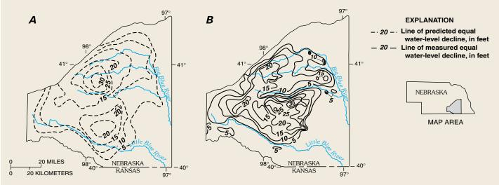
*Figure F–1.* (*A*) Predicted and (*B*) measured ground-water-level declines in the Blue River Basin from predevelopment to 1982. (Emery, 1965; Johnson and Pederson, 1983.)
