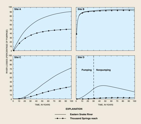
**Figure C–4.** Simulated losses to the Snake River resulting from pumping at well sites A to D. (Modified from Hubbell and others, 1997; reprinted with permission of the National Ground Water Association. Copyright 1997.)
