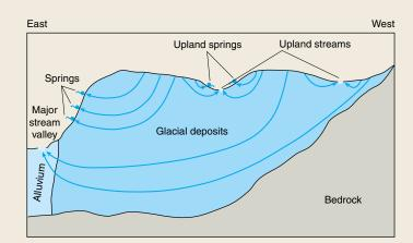
**Figure C–2.** Simplified hydrogeologic section for basin shown in Figure C-1 showing generalized ground-water-flow paths under natural conditions. Confining units and their effect on the flow system are not shown. (Modified from Morgan and Jones, 1999.)
