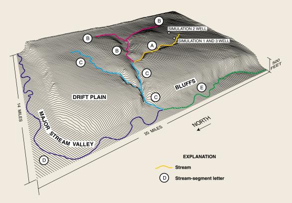
**Figure C–1.** Three-dimensional perspective view of a hypothetical basin typical of the Puget Sound Lowland showing topography, streams, and well locations for pumping simulations. (Modified from Morgan and Jones, 1999.)
