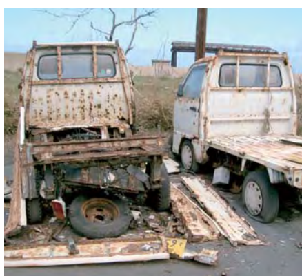
Cars Rusted and Broken Down Due to Volcanic Gas
