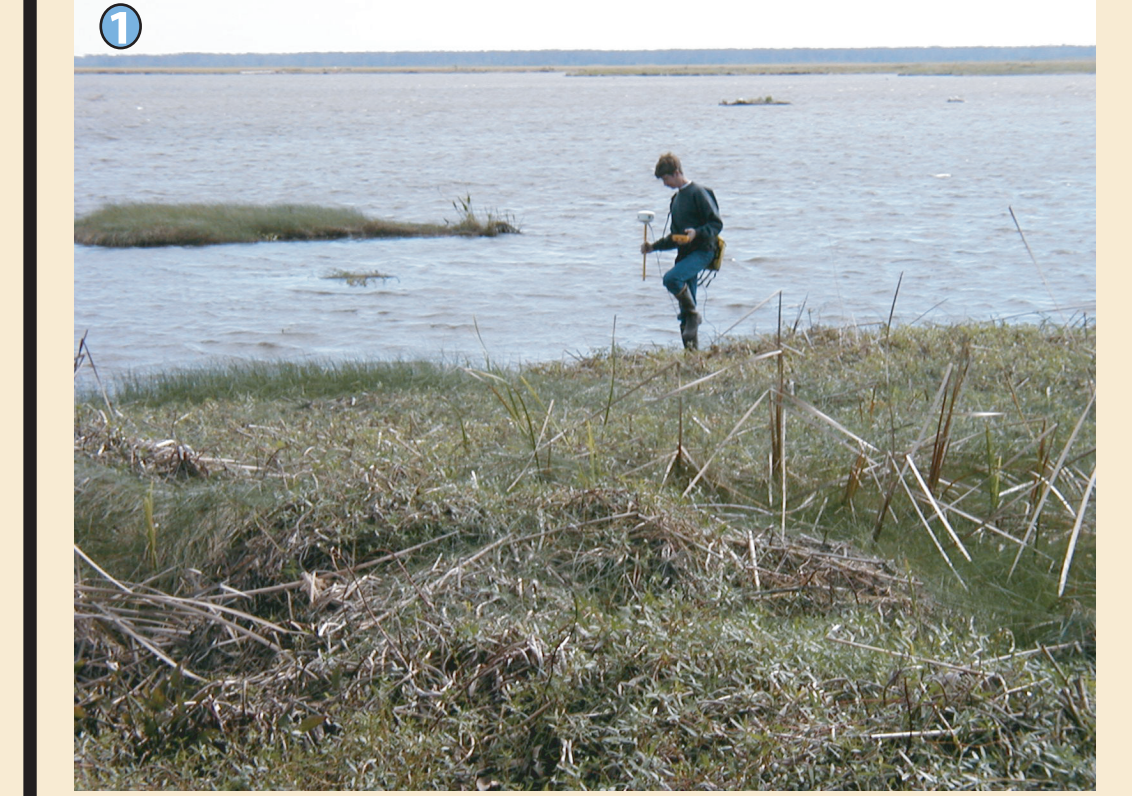
Acquiring Global Positioning System coordinates on marsh "island" in the middle of the new 175-acre pond. The island consists of ripped up, 0.5 m thick marsh mats resting on the old marsh surface. Pond depths ranged from 0.5 to 1.3 m. Photo taken facing the northeast.
