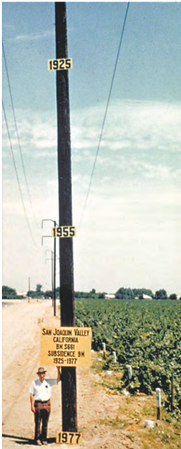
Figure 8. Approximate location of maximum subsidence in United States identified by research efforts of Joseph Poland (pictured). Signs on pole show approximate altitude of land surface in 1925, 1955, and 1977. The pole is near benchmark S661 in the San Joaquin Valley southwest of Mendota, California (from Galloway and Riley, 1999).
