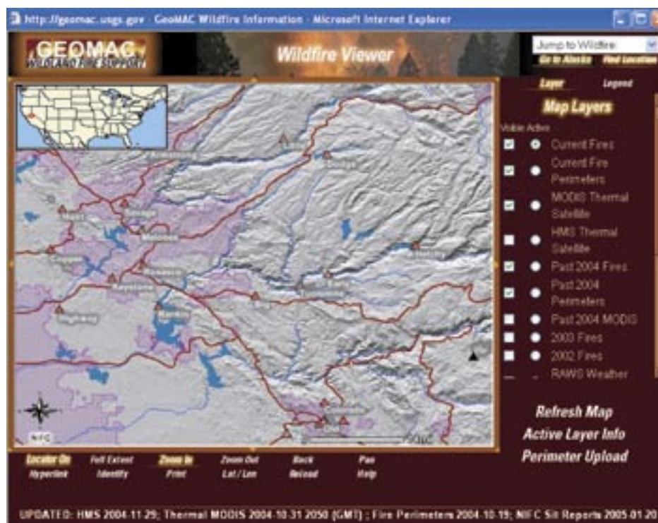
Figure 3: The GeoMAC Web site and mapping application customizes the dissemination mode and type of information supplied to both the general public and to firefighting practitioners
