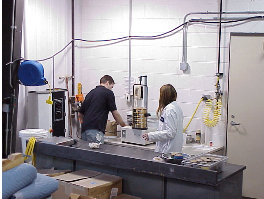
Figure 1 - Performing soil gradation tests in the GTI Soils Lab
