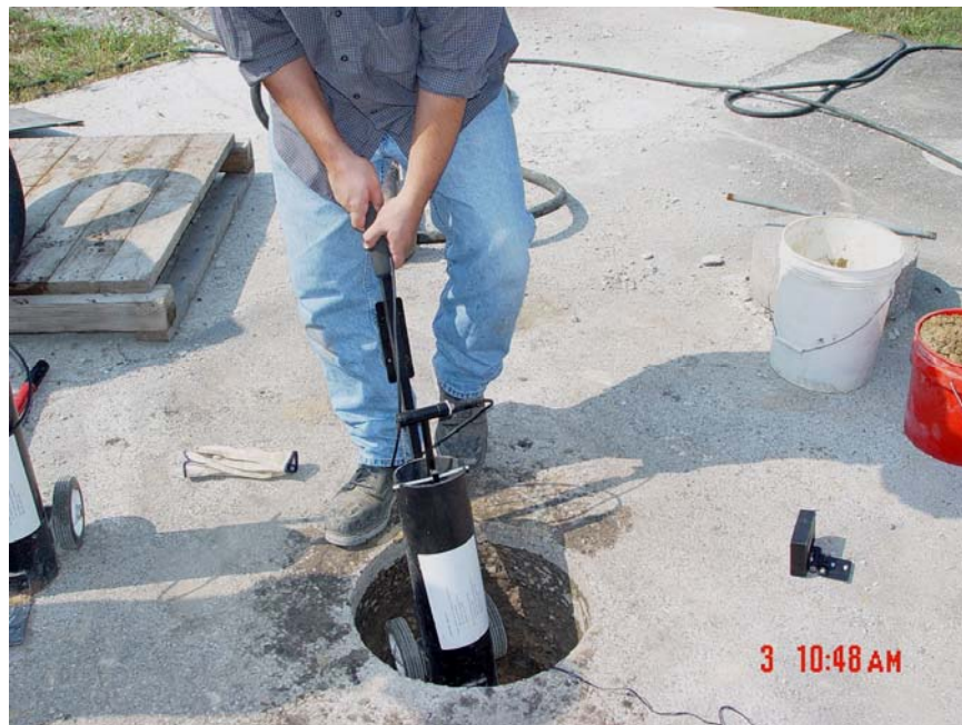
Figure 14 –Compaction measurements using the Clegg Hammer
