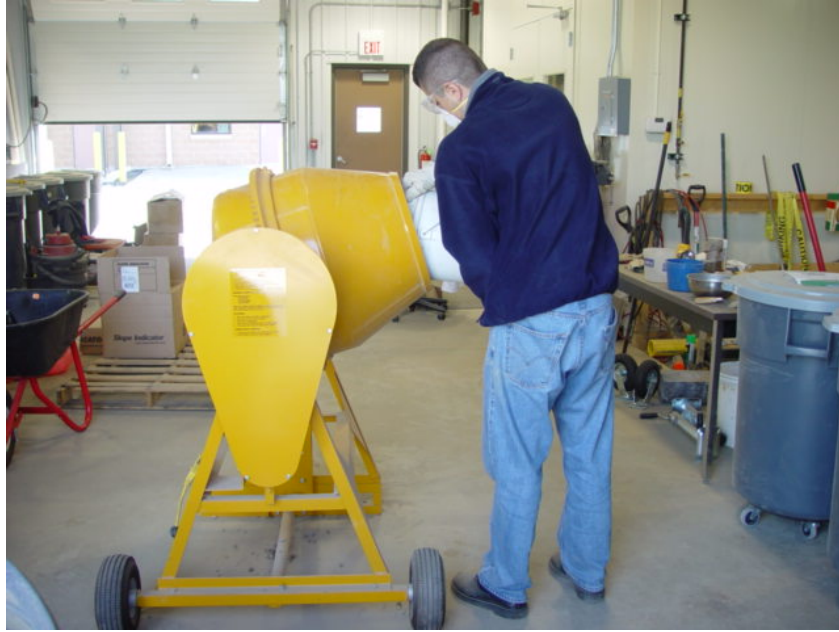
Figure 18 – Soil mixing procedure for uniform moisture content
