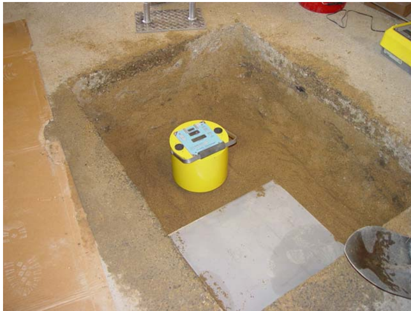
Figure 11 – Testing the devices with and without the rigid plate in the bellhole
