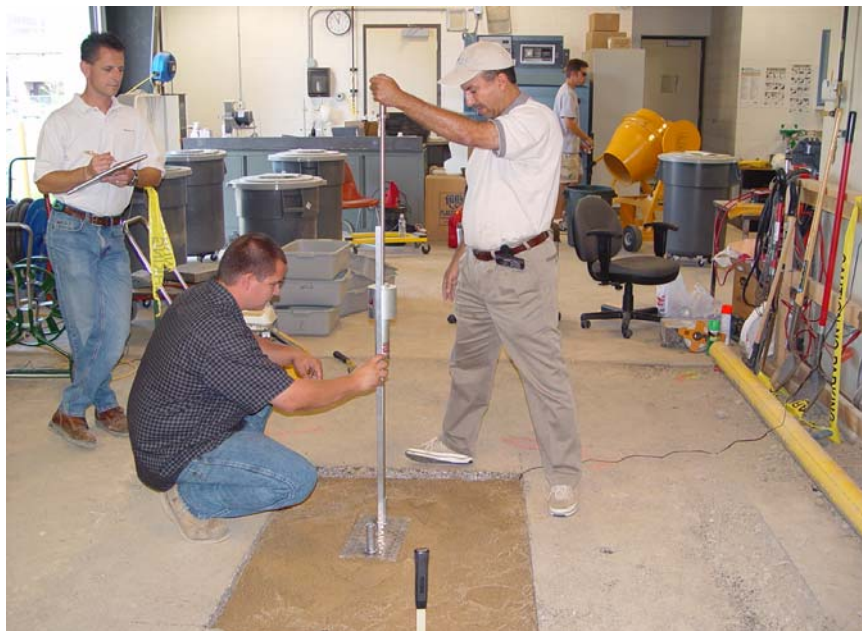
Figure 70 - The DCP test in the indoor bellhole section
