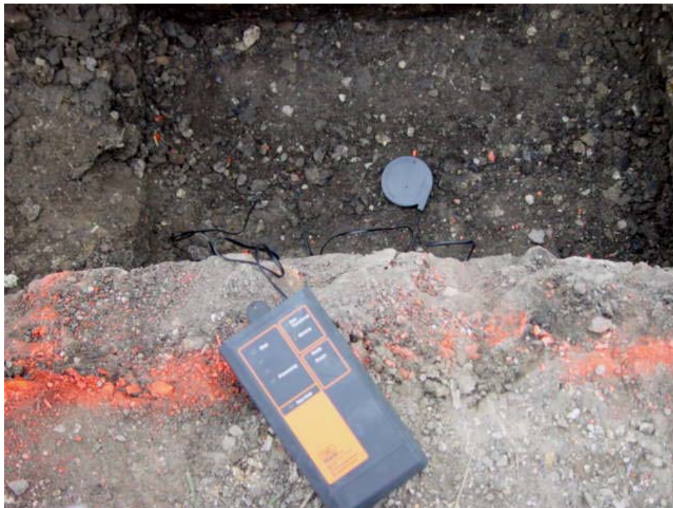
Figure 36 – The SCS sensor with the disk at the bottom of the trench
