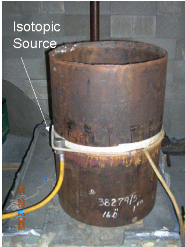
Figure 7. Photograph showing isotopic source used for double wall radiographs
