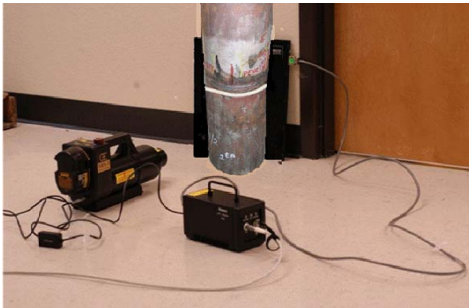
Figure 8. Pulsed x-ray source with Vidisco real-time imaging used for double wall radiographs
