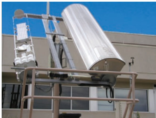
Prototype concentrator evaluation test bed contains prototype cell assemblies on right and variety of lens and mirror-based concentrator modules on left
