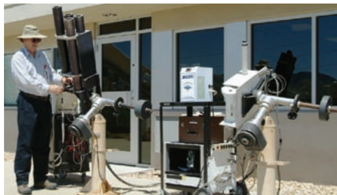
Test bed for calibrating primary reference cells
