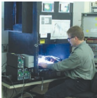
ISO 17025 accredited test bed for calibrating secondary reference cells
