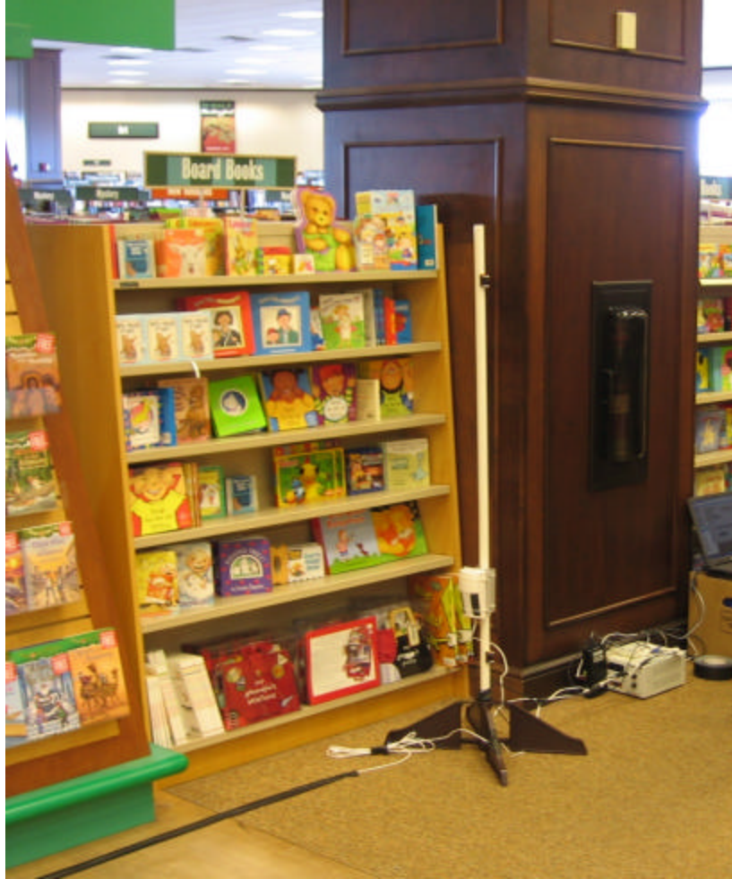
Figure 12: Detector Pole (with PIR Sensor) Position
