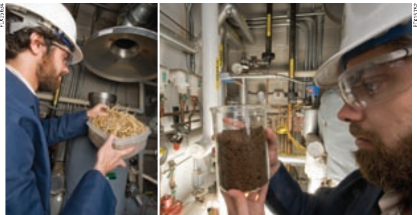
Researcher Noah Weiss feeds raw corn stover into a pretreatment reactor (left) and examines the product (right) after the reactor has extracted the hemicellulose as xylose.
