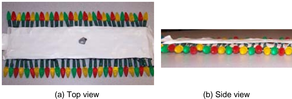
Figure 1. A mounted decorative light string prepared for testing.
