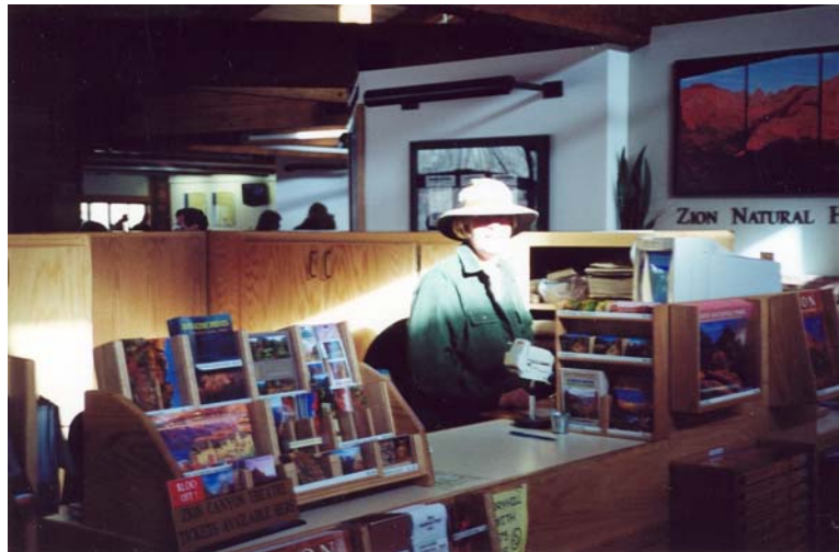
Figure 3-12 Zion bookstore checkout counter glare from clerestories
