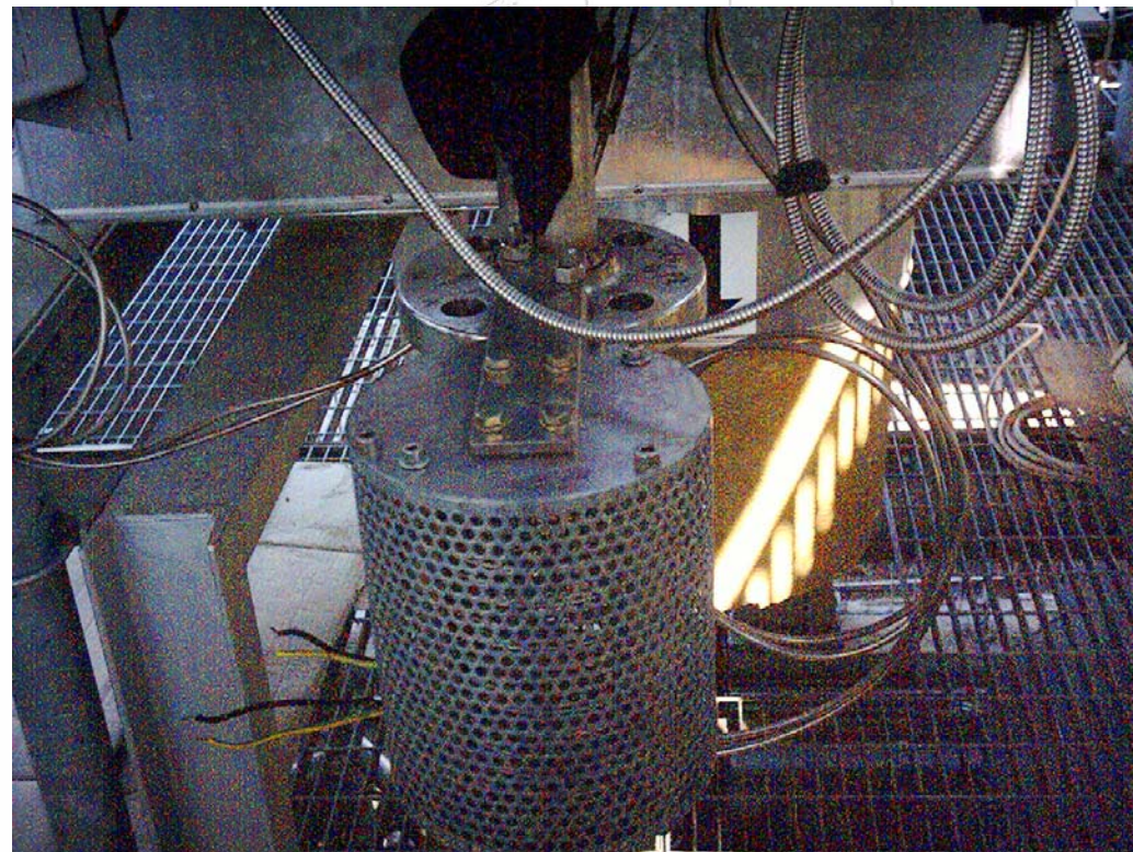
Test apparatus for comparison of pressure measurement with and without diaphragm seal (siliconic oil) and thermostatic drainage valve (joule effect operated)
