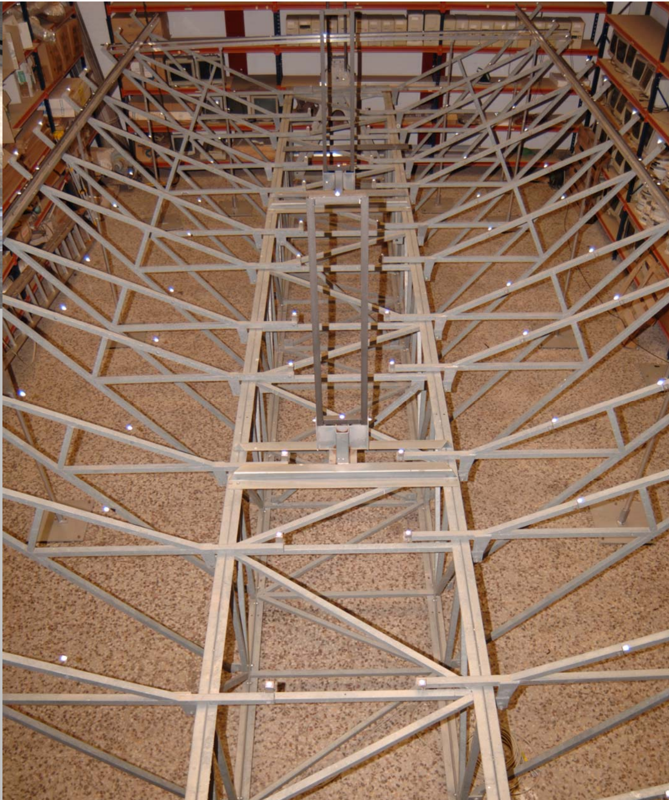
Top: tilting camera on shuttle Bottom: Scheme of the measurement configuration Right: Collector support structure with reflecting targets
