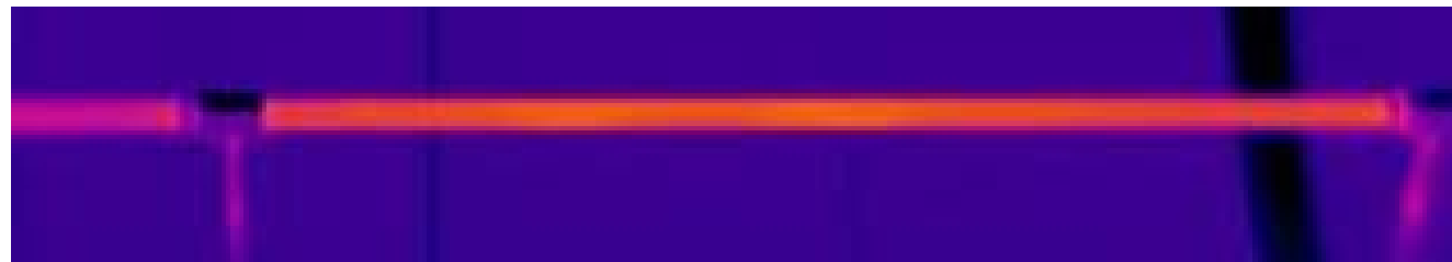
Infrared Image – Not Tracking (Glass Temp. 124°C-141°C )
