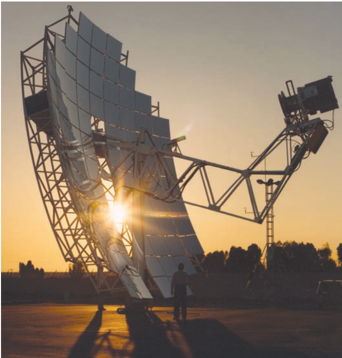
DOE national labs assist industry in improving dish-Stirling engine systems. Early in 2008, a 25-kilowatt (kW) Stirling Energy System dish set a new solar-to-grid system conversion efficiency record of 31.25%, generating a net electrical output of 26.75 kW.
