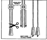
Figure 4. Making Pull-Cords Safer
