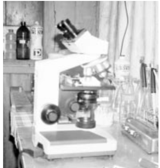
Figure 1.4. A small laboratory microscope requires only moderate use of a 30 watt light. It is essential equipment for diagnosis in the field.
