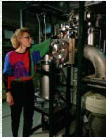
NREL's molecular beam mass spectrometer helps industry partners define process conditions in real time and minimize process emissions
