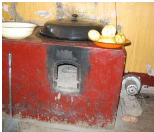
An oven equipped with electric fan (on floor).
