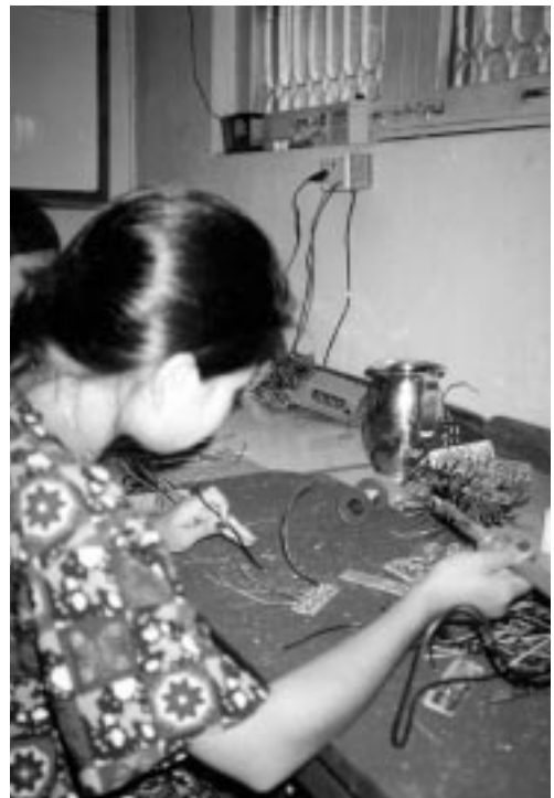
Figure 3.7. A worker assembles inverters and controllers at Lotus Energy plant in Nepal.
