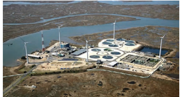
The Atlantic City Utilities Authority Wastewater Treatment Facility features the 7.5 MW Jersey-Atlantic Wind Farm and a 500 kW solar project. When dedicated in December 2005, the wind farm was the first in New Jersey, and the solar project was the second largest in the state.
